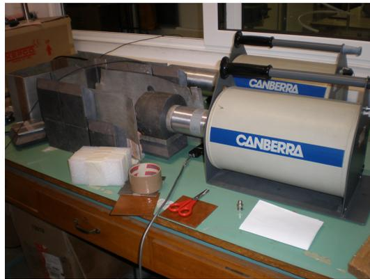
Figure 2.15: the 16% HPGe detector used for the measurement of the foils activity
