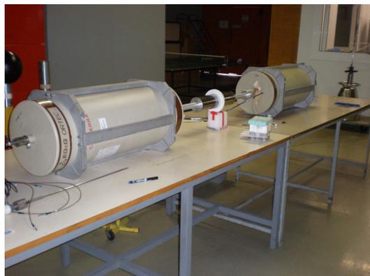
Figure 2.14: the 2x100% HPGe detectors used for the erbium pellet activity measurement
